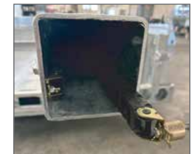
TONGUE WIRING IN CAT TRACK (No need to unplug tongue)
