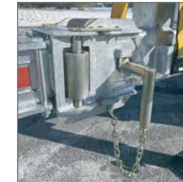
MEGA-ROLLER SYSTEM TONGUE SECUREMENT (w/Self-Securing Securelock™)
