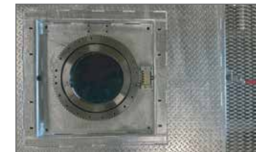
OVERSIZED 20" SLEWING RING (Lockable at every 3 degree interval)
